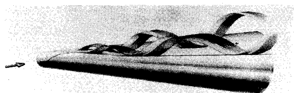
Fig. 18 Conceptual drawing of new model of boundary-layer separation on a blunt cone at angle of attack.
